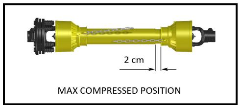
A driveshaft too long may cause structural damages to the tractor and machine. If the driveshaft is too long, it may be adapted by removing it and shortening the tubes according to the instructions provided by the manufacturer in its use and maintenance manual.
