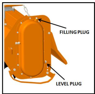
Check the oil level every 50 hours, making sure it reaches the level plug on the transmission cover.
