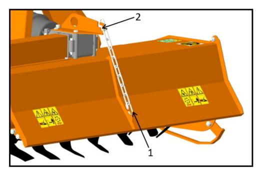
• to raise the rear board, reduce the number of chain links in tension. This operation, together with the increase of the tractor ground speed, allows to have a coarser soil texture;
