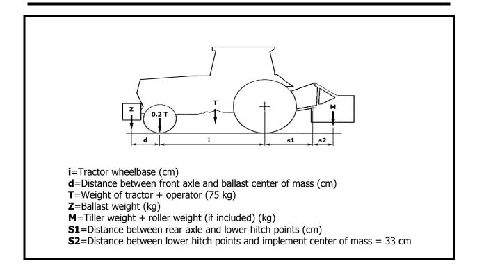
If the Tiller is combined with other machines (fertilizers spreaders or seeders), the ballast check must be done considering:
