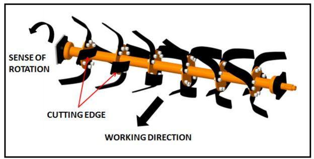
Periodically check the tightness of screws and nuts, and tighten if necessary.
