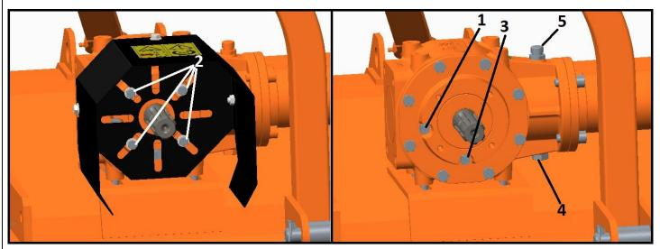
If the oil level is below the line of the level plug, it's necessary fill up oil till restore the correct level.
