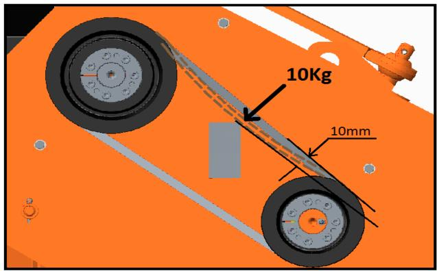
If the deflection is about 10 mm, the tension is correct. If is not so, proceed with the adjustment in the following way (see picture below):
