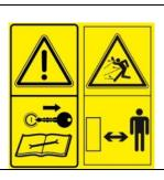
Disengage the PTO, turn off the tractor engine, remove the key and ensure that all rotating parts have stopped before approaching the implement.
