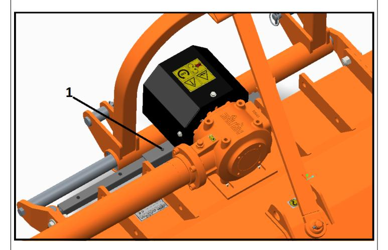
In case of configuration with hydraulic cylinder, the side adjustment of the frame is effected by actuating the cylinder directly by the hydraulic control system of the tractor, after performed the connection of the machine hydraulics to the tractor.
