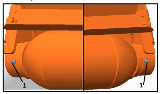
To perform lubrication, inject grease into the nipples (1) and (2), located on the upper part of the roller bearing supports (see pictures).
