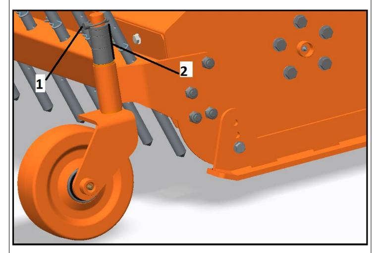
Depending on the different position of the spacers on the shaft, it is possible to set five different cutting heights: 70-76-89-114 and 145 mm.
