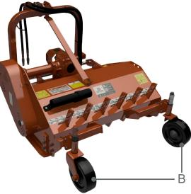
The working height of the machine is determined by the vertical position of the rear roller "A" or swivel wheels "B" (optional).
