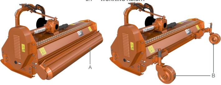
The working height of the machine is determined by the vertical position of the rear roller "A" or swivel wheels "B" (optional).
