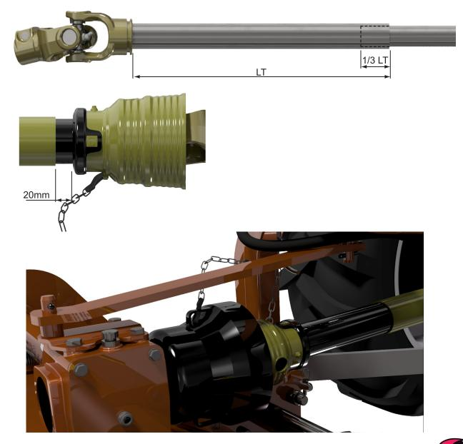
Insert the first hub of the cardan shaft onto the flail mower PTO, holding the safety pin or safety collar pressed. Release the pin and retract with the cardan until the pin itself engages in the relevant seat with an audible "clack".
