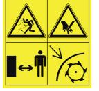
Warning Danger of flying objects During functioning, the machine can project material from the rear part: make sure that animals and persons are at least 50 metres from the machine.
