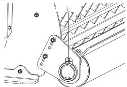
GREASING LATERAL TRANSMISSION JOINT (Every 20 working hours)
