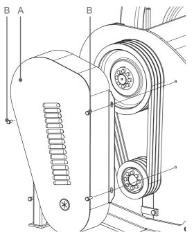
Frequently check the state of wear of the belts and replace the entire set if one or more result deteriorated.
